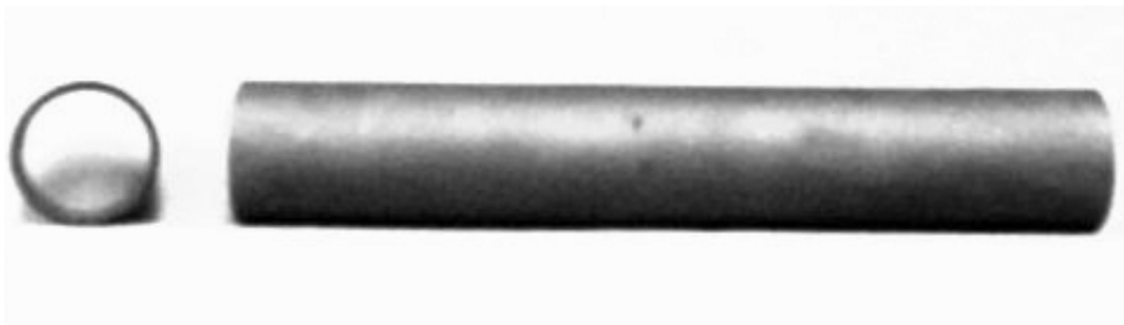
Figure 5.17: Photograph of a sintered 95% dense \text{La}_{0.5}\text{Sr}_{0.5}\text{CoO}_{3-\delta} tube with a length of 13 cm.
